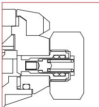
**1** Crown equipped with double O'ring for perfect water-resistance
