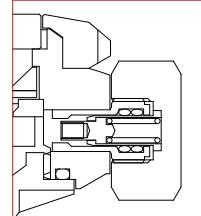
1 Crown equipped with double O'ring for perfect water resistance
