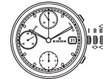
Some Edox Chronograph watches have a tachymeter scale. With this scale it is possible to measure the speed. The distance is 1 km. To measure the elapsed time press the start/stop button when the vehicle (power-boat) passes the starting and the final point or target. The figure shown by the hand on the tachymeter scale indicates the average speed in kilometers. If for instance a car covers a 1 km distance in 30 seconds, you can consider it to an average speed of 120 km per hour.
